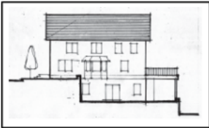
Inappropriate: Clearing the site; using cut and fill and retaining walls.
